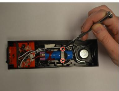
Identify the two Phillips (Length-5/16", Head-1/8") screws holding the battery in place and remove them using a #1 screwdriver.
