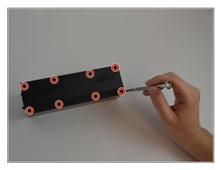
Flip the device upside down and remove all eight Phillips (Length-3/8", Head-1/8") Screws using a standard #1 Phillips screwdriver.
