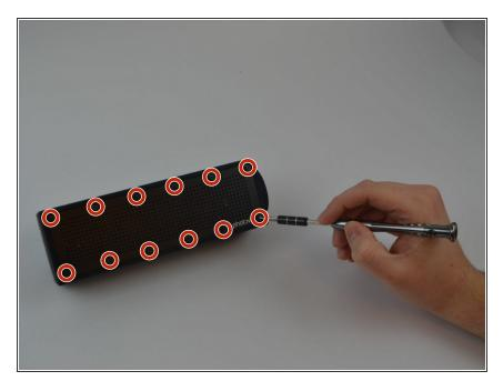
Unscrew all twelve Hex Head 1.5 (Length-3/8", Head- 1/8") screws using a 1.5mm hex screwdriver.
