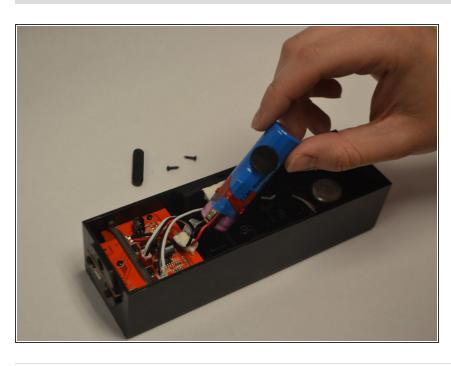
Remove the ICR18650-26M battery from its position by pulling upwards and out of the casing.
