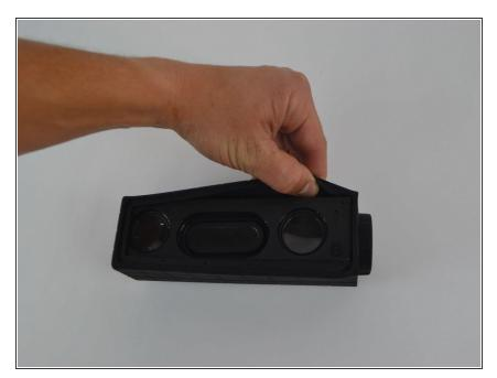
Remove the rubber casing by using your fingers to pull off. Be sure not tear or rip rubber casing.
