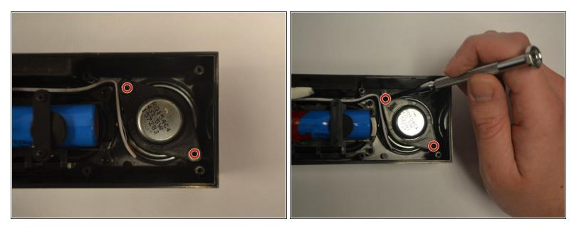
Identify the two Phillips (Length-5/16" Head-1/8") screws holding the speaker in place and remove them.
