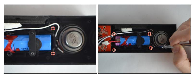
Identify the four Phillips (Length-5/16", Head-1/8") screws holding the speaker housing (below the battery) and remove them.
