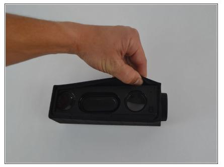
Remove the rubber casing by using your fingers to pull off. Be sure not tear or rip rubber casing.
