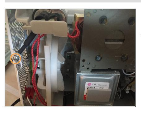
Remove the screw holding the capacitor ground on the left side of the oven. and set the capacitor aside.
