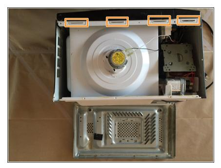
Lift the vented metal plate from the back side at an angle until the clips on the front side by the oven door are no longer holding the plate. Set bottom plate aside and the oven's contents are accessible.
