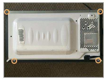
On the BACK side of the oven you'll find a T8 torx screw on each corner; remove all four.
