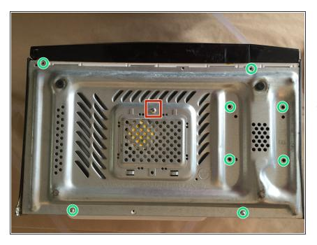
On the bottom of the microwave you'll find 9 more phillips screws. Remove the four on the top and bottom of the casing, and four more on the right side which are holding the transformer to the inside of the case. Leave the last screw, which is located in the raised rectangle in the middle of the bottom panel,
