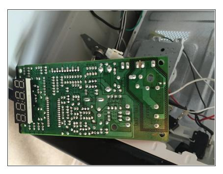
The PCB for the keyboard and the LED display has two phillips screws hidden between on-board components. The board also has several connectors that cannot be removed reliably without jeopardizing the functionality of the oven, so it is recommended to leave the board connected unless it must be replaced.
