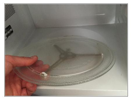
Before beginning with the disassembly, open the microwave oven door and remove the food plate and the turntable it sits on so they aren't sliding around during the rest of the teardown.
