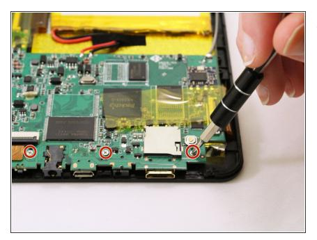
• Use a PH00 screw driver to remove the three 4 mm screws holding the motherboard down.
