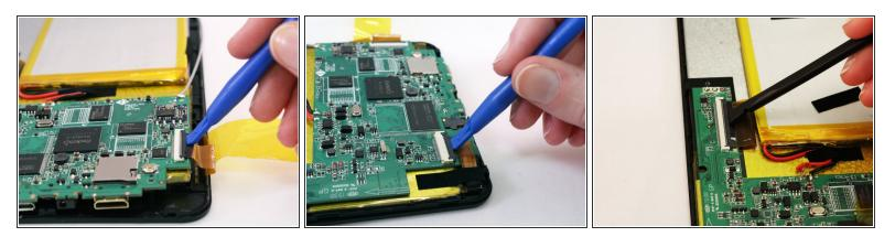
• Lift all three ZIF connectors to disconnect the ribbon wire.
