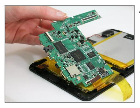
• Lift the motherboard off the device.
