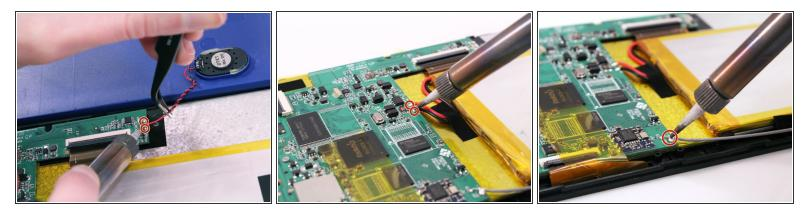
• With the soldering tool remove the speaker wires, battery wires and gray wire that are connected to the motherboard.
