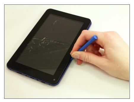
• Use the blue opening tool to pry the tablet open.
