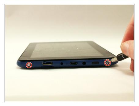
Remove both 4 mm screws from the top of the tablet using a PH00 screw driver.
