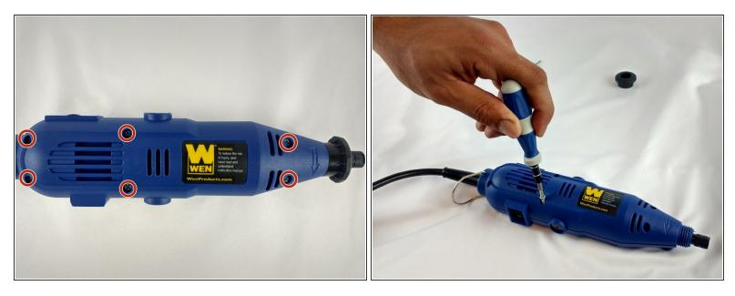
Unscrew the six 8mm PH2 screws.
