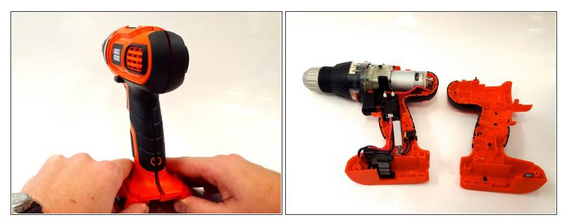
• Carefully remove the plastic drill casing by pulling it apart.
