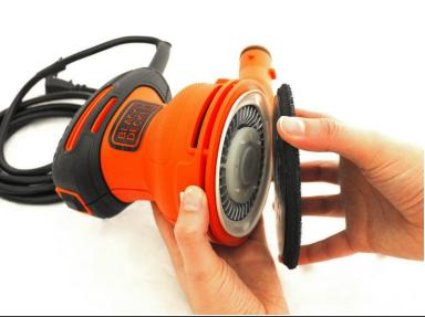
Once all screws and washers have been removed, hold the hook and loop system and separate it from the device.
