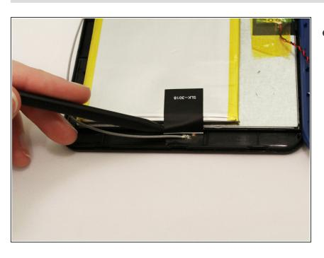
Use a spudger to remove the black tape from the battery.
