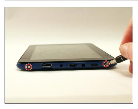
Remove both 4 mm screws on the top of the tablet with a PH00 screw driver.
