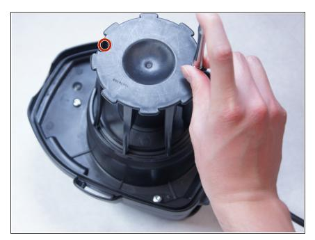
Use a 3.5 mm hex key to remove the two screws securing the filter cage.
