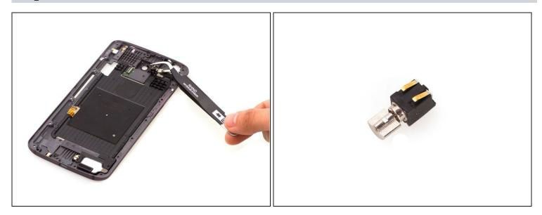
• The vibrator is only fastened by the plastic bracket.
