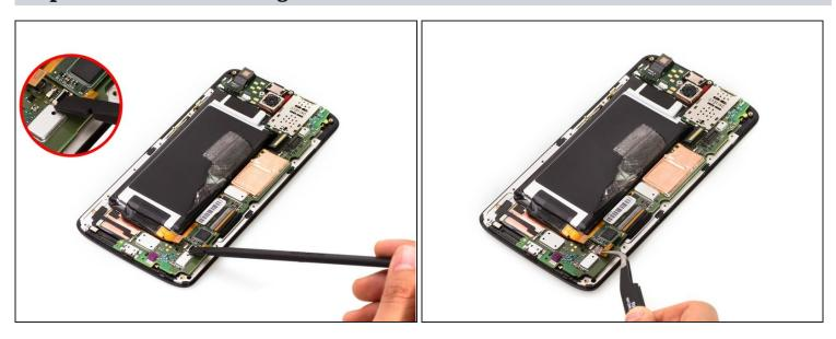
• The LCD assembly has two connectors, here is touchscreen connector.
