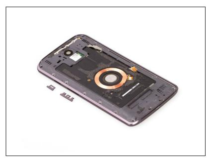
After middle frame's separating from the rest of parts, side buttons are loose and easy to remove.
