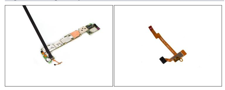
• With this sensor flex, you can wave your hand on the top of the screen to wake up the screen.
