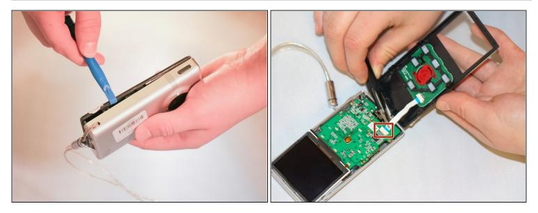
• With the plastic opening tool, gently pry the front casing away from the device by carefully running the tool around each edge and lifting.
