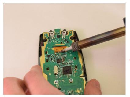
Use a soldering iron to loosen the solder that connects the screen strip to the back of the motherboard. If it does not loosen easily then try using a soldering remover wick.
