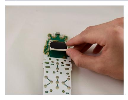
• Use a spudger or your hand to remove the screen from the motherboard. It is glued down.
