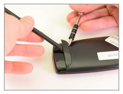
Remove the small plastic cover beneath the plastic LED housing by using a <u>3.0 flathead</u> screwdriver and a spudger to pry it off. It is glued to the case. If you are having trouble removing it try applying some heat to loosen the glue.
