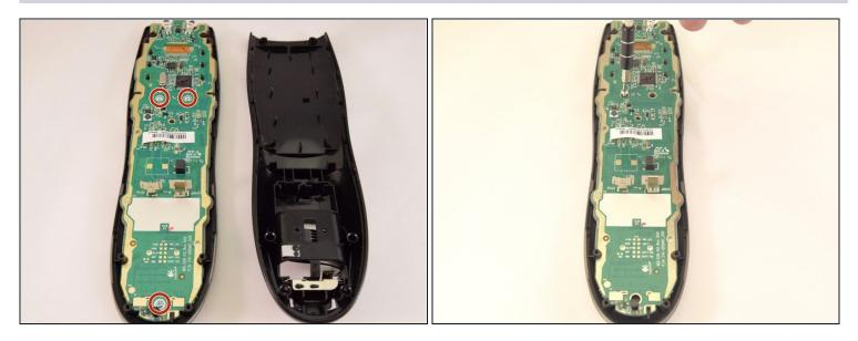
• Using a J0 screwdriver remove the three 5mm screws holding the motherboard to the front face. Two are located just below the processor in the middle of the device and the third is located at the very bottom.
