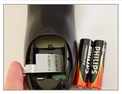
• Remove the batteries using the silver pull tab.
