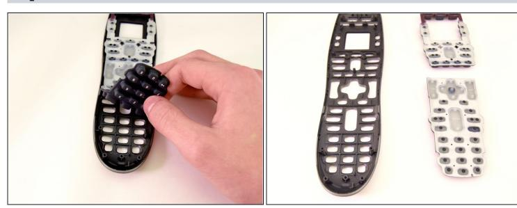
• Peel away both the upper and lower sets of buttons using your fingers.
