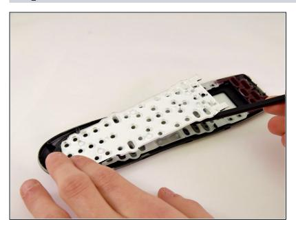
Using a spudger, gently pry the bottom retaining place from the front case.
