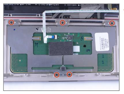
• Unscrew the five 2.3 mm screws using the PH000 screw head.
