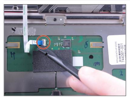
Lift up the latch using the nylon spudger.
