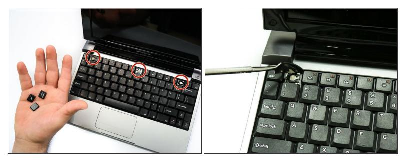
To take off the Keyboard there are three tabs at the top of the Keyboard in the locations shown in the picture that you must press and unclip. They are located behind each of the keys that are removed.
