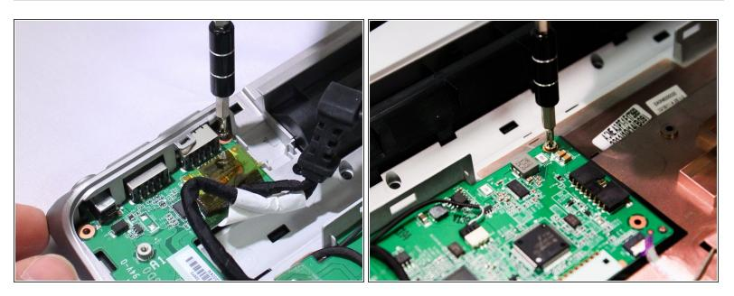
• Remove the two 2mm long phillips head screws that are holding down the motherboard.
