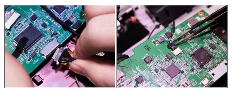
• Disconnect the two wires that attach to the screen from the motherboard.
