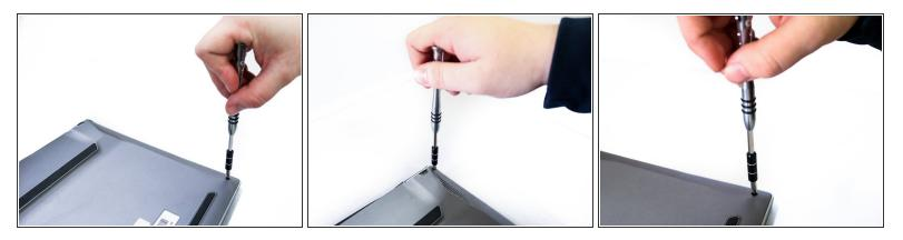
• Flip over the Lapdock and remove the four 3.5mm long phillips head screws from the bottom.
