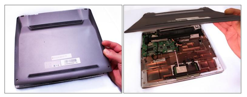
Use a plastic prying tool to take off the bottom case. Make sure that all of the clips are unclipped before trying to remove the case.
