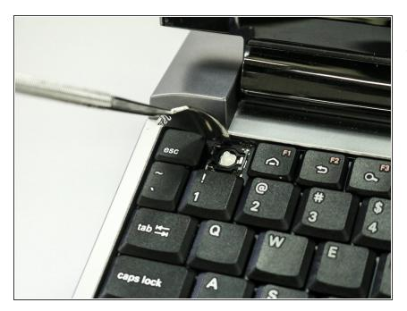
You can use a small metal spudger to depress each tab to avoid scratching the keyboard.
