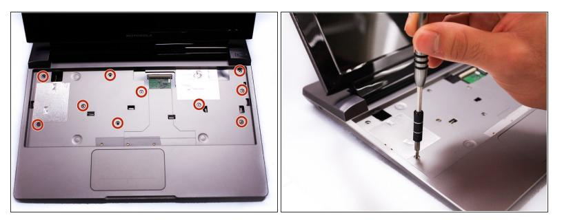
After we remove the Keyboard, you can clearly see the screws under it. Remove the ten 3mm long phillips head screws.
