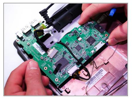
• The motherboard and phone adapter cable should both be free from the lapdock.
