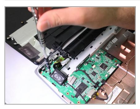
Remove the two 2mm long phillips head screws from the left speaker and move it away from the motherboard.
