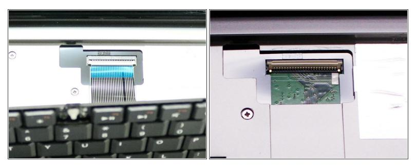
• Flip up the ZIF connector holding the ribbon cable on the contact as shown in the two pictures and then gently disconnect the ribbon cable.
