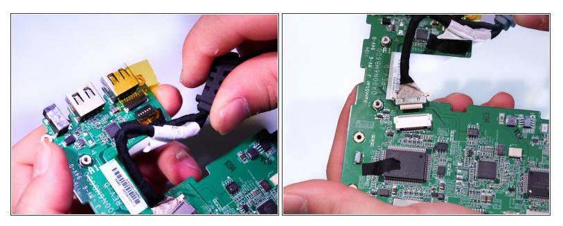
• Unplug the two phone adapter cable connections to the motherboard.
