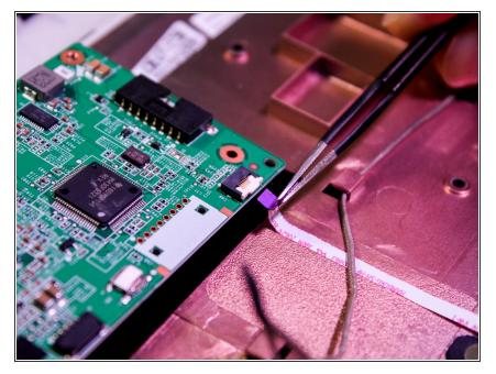
Disconnect the ribbon cable that attaches to the trackpad from the motherboard.
