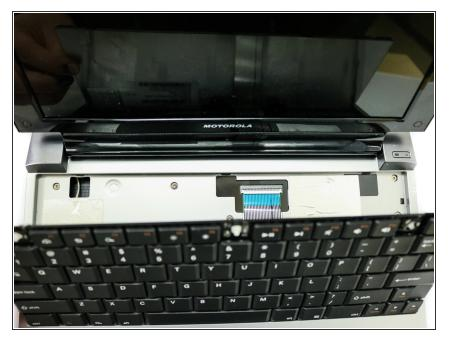
• Lift up keyboard so that you are able to see the ribbon cable connected to the contact.
