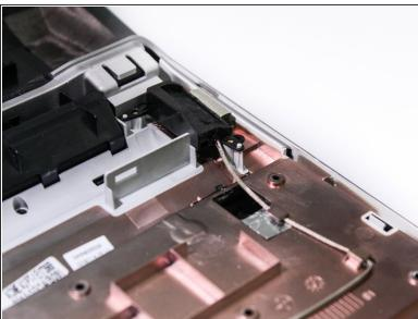
Remove the two 2mm long phillips head screws from each speaker.
