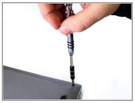
Flip over the Lapdock and remove the four 3.5mm long phillips head screws from the bottom.
