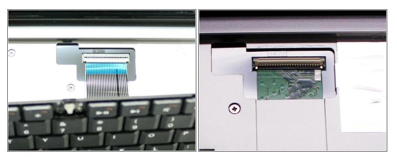
• Flip up the ZIF connector holding the ribbon cable on the contact as shown in the two pictures and then gently disconnect the ribbon cable.
