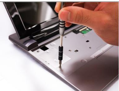
After we remove the Keyboard, you can clearly see the screws under it. Remove the ten 3mm long phillips head screws.
