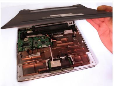
Use a plastic prying tool to take off the bottom case. Make sure that all of the clips are unclipped before trying to remove the case.
