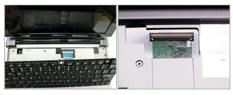
Flip up white clip holding the ribbon cable on the contact as shown in the two pictures and then gently disconnect the ribbon cable.
