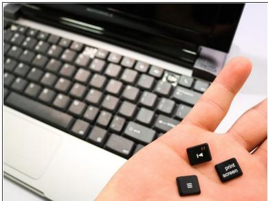
To take off the Keyboard there are three tabs at the top of the Keyboard in the locations shown in the picture that you must press and unclip. They are located behind each of the keys that are removed. You do not need to remove any keys to unclip the keyboard.
