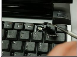
You can use the a small metal spudger to depress each tab to avoid scratching the keyboard.
