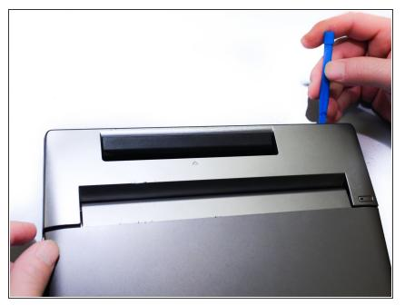
Now flip the lapdock back over. Using a plastic prying tool, unclip and remove the small plastic cover at the top of the lapdock.
