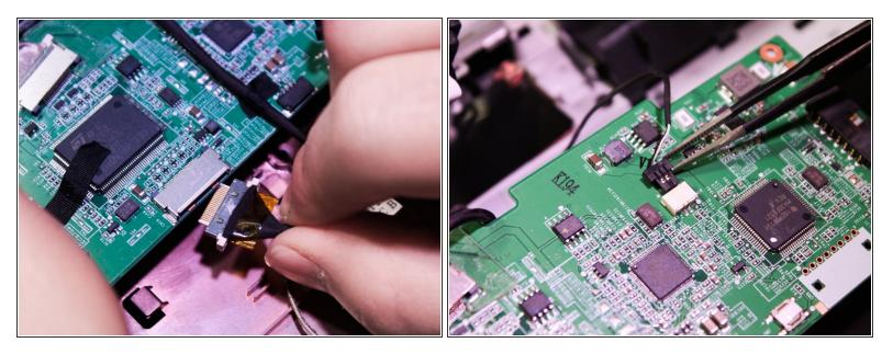
• Disconnect the two wires that attach to the screen.
