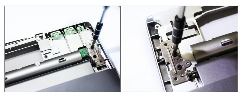
• Remove the four 3.5 mm long phillips head screws from the two screen flanges holding the screen.
