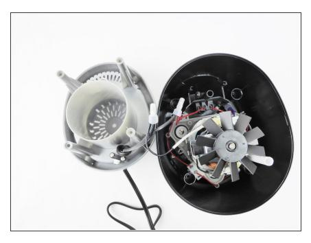
Remove the gray base by lifting upwards and placing to the side.
