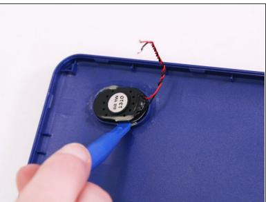
• If needed use a plastic opening tool to remove speaker from the speaker port on the tablet.
