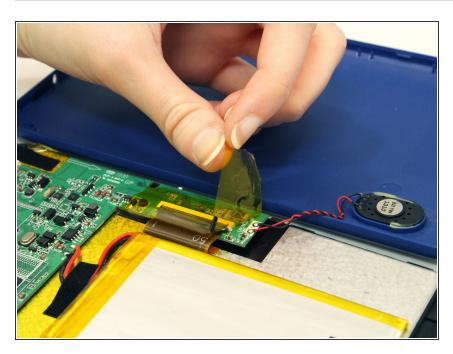
Pull back the protective tape from the two wires that connect the speakers to the motherboard.
