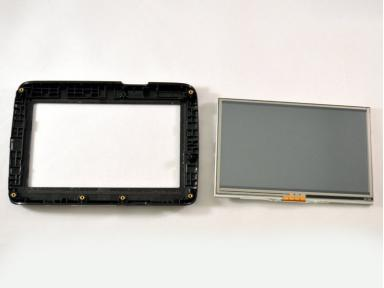
Pry back on the plastic shell surrounding the touchscreen and remove the screen.
