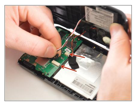
Disconnect battery and speaker cables from the motherboard at indicated places.
