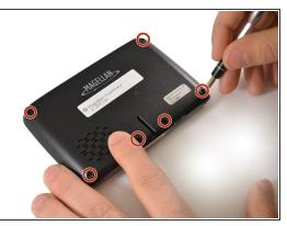
Turn the GPS over on its backside and remove the six 3 mm Phillips #1 screws.
