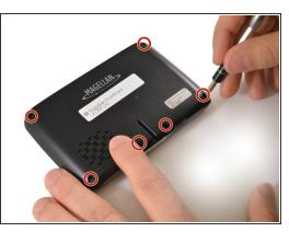
Turn the GPS over on its backside and remove the six 3 mm Phillips #1 screws.
