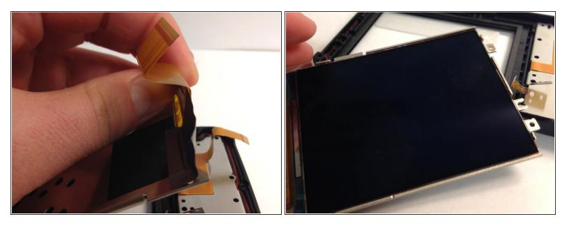
• Pull the LCD screen from the plastic frame after removing all of the screws.
