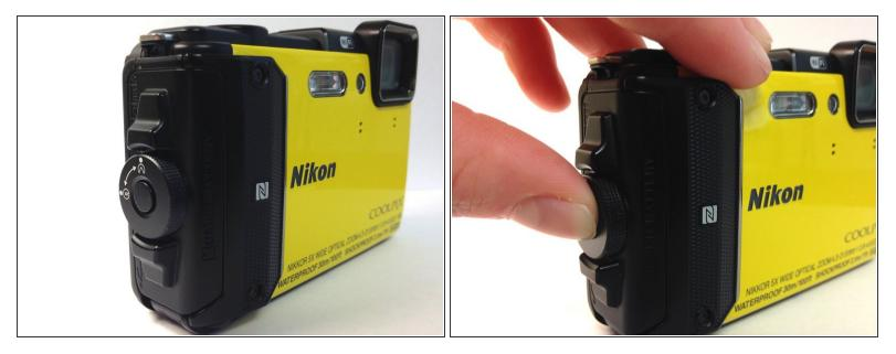
Using your thumb and pointer finger, open the card/battery hatch by pressing the center button of the wheel and turning the entire wheel to the left.
