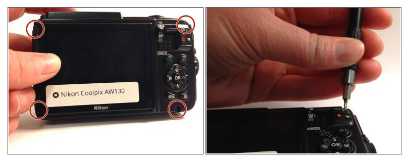
Using the T5 Torx screwdriver, remove all four 4mm screws.
