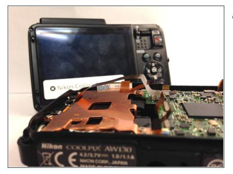
• Carefully remove the back cover from the camera body.
