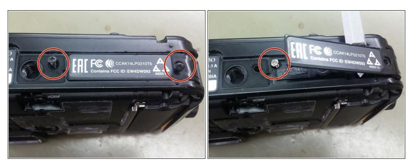
Remove two Philips screws from the bottom cover, lift gently the cover and remove the single Philips screw under it.
