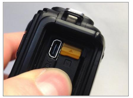
Push the yellow battery/charger compartment tab up using your thumb nail.
