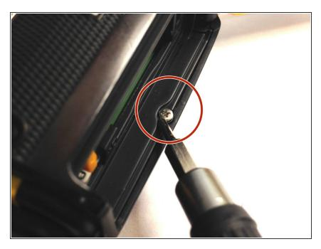
Using a Phillips #000 screwdriver, remove the single 3mm screw found inside the battery/charging compartment.
