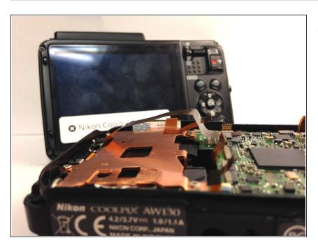
Carefully remove the back cover from the camera body.
