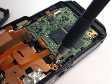
• Using a Phillips #000 screwdriver, remove all 8, 4mm screws on the motherboard.
