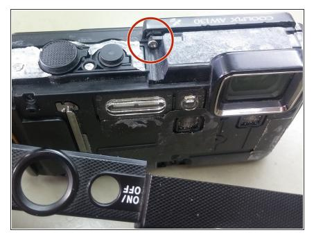
Remove the upper cover (connected by glue) and unscrew the single Philips screw.
