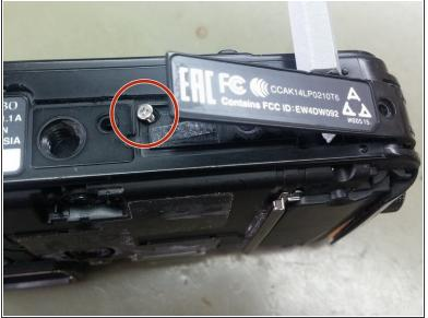
Remove two Philips screws from the bottom cover, lift gently the cover and remove the single Philips screw under it.
