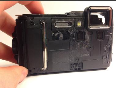
Using the metal spudger tool, pry the colored face from the camera body.
