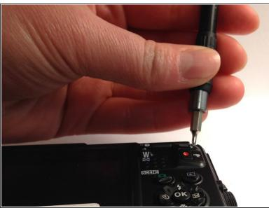
Using the T5 Torx screwdriver, remove all four 4mm screws.
