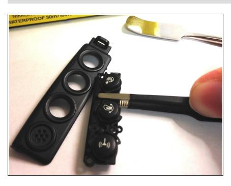
Using tweezers from the precision tweezer set, remove the buttons from the larger plastic piece.
