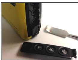
Using the spudger, pry the plastic button face from the camera body.
