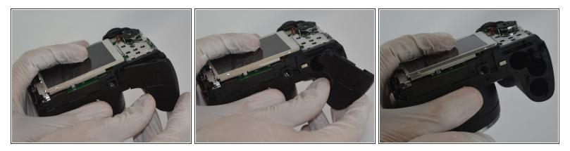
• Once the back plate is removed twist the battery cover clockwise and it should easily dislodge.
