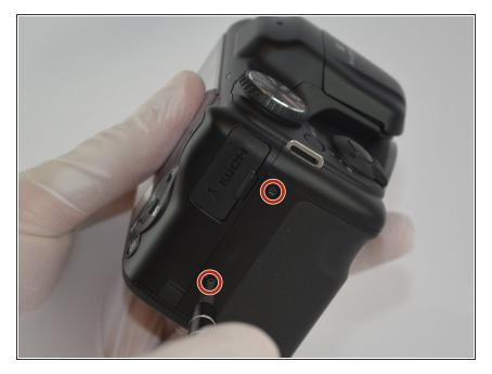
Use your Philips Head Screwdriver to remove the M3 x 4mm screws from the right side of the device as indicated by the pictures.
