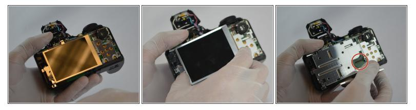
• Gently pull the tab out of the motherboard and then the LCD screen should easily be removed.
