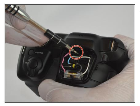
Fold the lid down in order to access and remove the final M3 x 4mm screw using your Philips Head Screwdriver.
