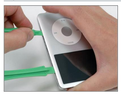
Remove the plastic opening tool from the top corner and insert it into the seam between the front and back of the iPod, leaving at least 1.5 inches of space between the two tools (as done on the other side).
