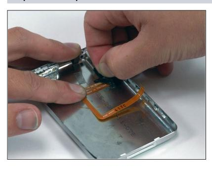
Use one hand to hold the orange ribbon cables in place, and peel up the black tape securing the cables to the rear panel with your other hand.
