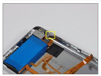
Now to repair the damage caused by liberating the internal parts of the iPod Classic! It is highly likely that at least one of the metal clips in the rear panel has been bent upward. These clips must all be pointing downward in order to reinstall the rear panel.
