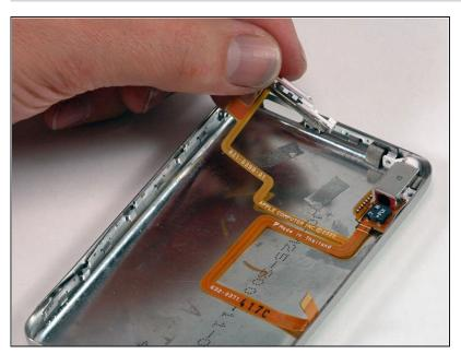
Lift the hold switch free from its housing on the rear panel. Don't remove the hold switch completely at this time, because it is connected to the same cable as the headphone jack.
