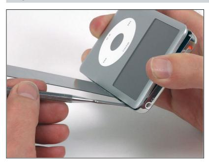
Gently wiggle the metal spudger down so that it is all the way in the rear panel.
