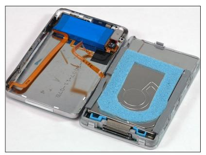
Place the rear panel next to the iPod, being careful not to strain the orange headphone jack cable.
