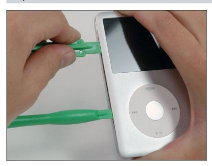
Insert another plastic opening tool into the seam between the front and back of the iPod, leaving at least 1.5 inches of space between the two tools.
