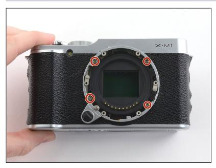
• Remove the four 4.3 mm screws securing the sensor to the front case.
