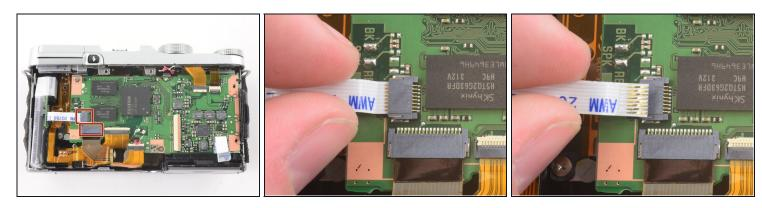
• Use two fingers to remove the two ribbon cables in the bottom left corner of the motherboard.
