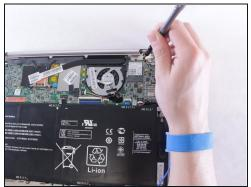
• Unscrew the two brackets using the Phillips Head #0.
