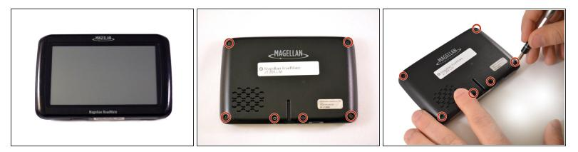
• Turn the GPS over on its backside and remove the six 3 mm Phillips #1 screws.
