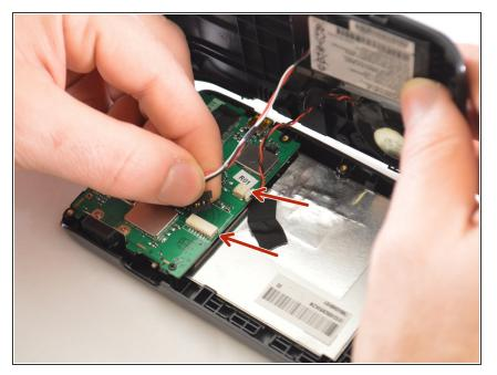
Disconnect battery and speaker cables from the motherboard at indicated places.
