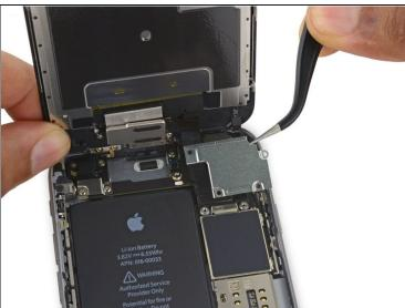
• Remove the display cable bracket.
