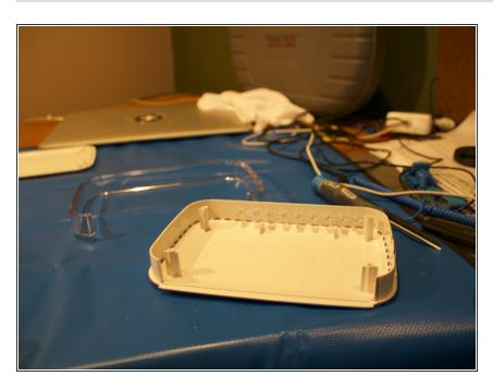
After remove the motherboard. The top cases of the Router.
