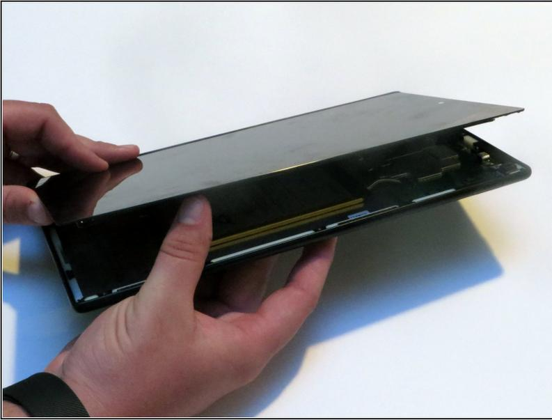
**⚠** Do not completely remove the screen yet as there is a ZIF connector connected.
