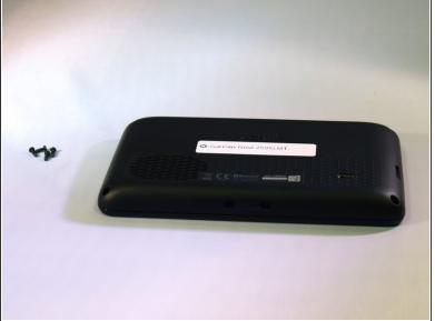
• Using the t5 screwdriver from the iFixit Pro Tool Kit, remove all four 5.6mm screws placing them safely on the table.
