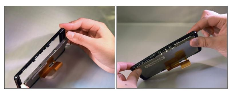
Place new screen in proper position, with the ribbon facing downward.
