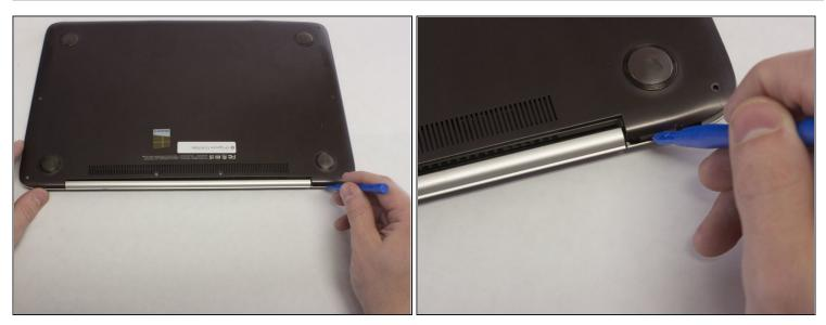
Use the plastic opening tool to lift the back case off.
