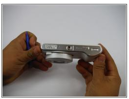
Face the camera towards you, then rotate it such that the battery door is facing up and to the right.
