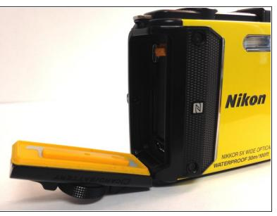
• You should feel the door begin to loosen. Carefully pull the hatch open.
