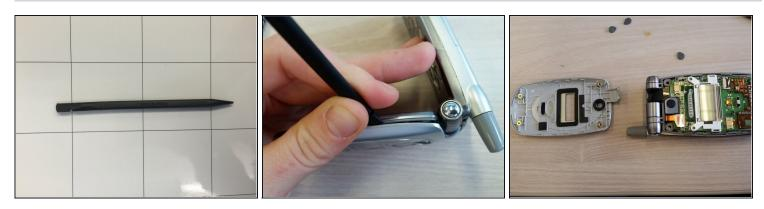
• Carefully pry front cover of cellphone off with flat end of nylon spudger.
