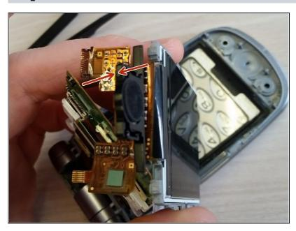
Attach new screen to circuit board. To reassemble your device, follow these instructions in the reverse order.
