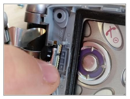
Use fingers to slide camera out of slot.
