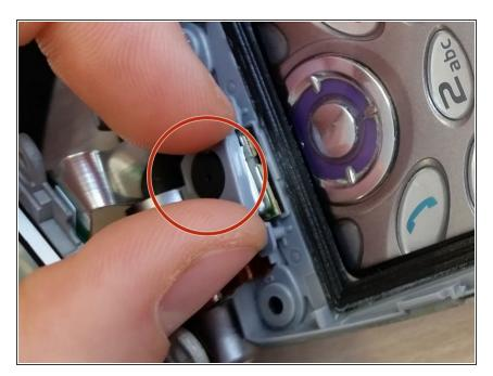
Pull off gray cover with black circular camera piece at the bottom of the screen.
