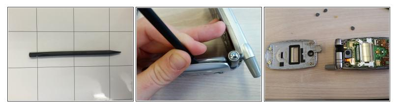
• Carefully pry front cover of cellphone off with flat end of nylon spudger.
