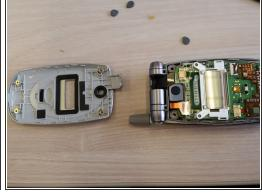
Carefully pry front cover of cellphone off with flat end of nylon spudger.
