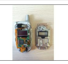
• Use a plastic opening tool to separate the inner metal cover from the circuit board. Apply pressure to remove the piece.
