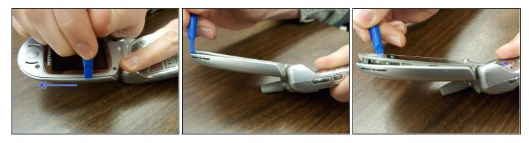
• Use a plastic opening tool to separate outer shell from metal interior cover by sliding it along the crease in the case.
