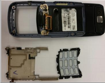
• Lift up the tan circuit board holder to separate it from the device.
