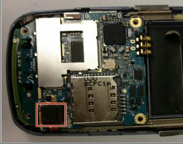
With care, lift up the connector located at the bottom left of the phone, as demonstrated in the accompanying image.
