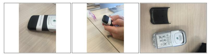
• Remove the back cover of the phone by pushing downwards with your thumbs.
