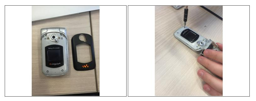
• You now have access to the fours screws that hold the front of the phone together. Remove the four screws.
