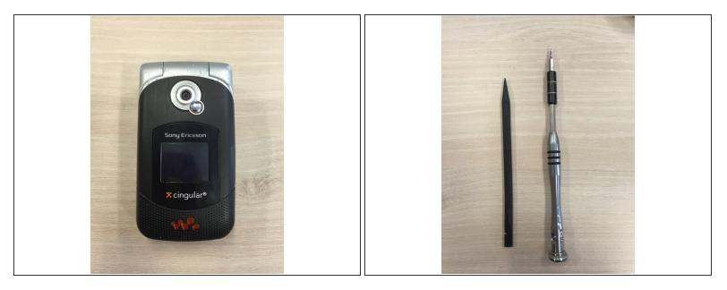
• The tools you will need for this step is the prying tool and the T6 Torx screwdriver.
