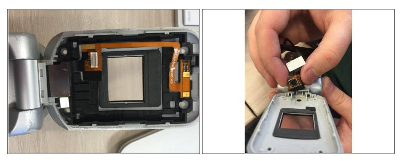
Now you have access to the camera, which is the silver plate at the bottom of the phone. Remove the camera and replace with a new camera.
