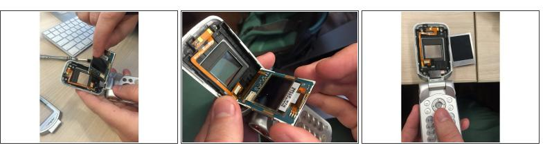
Use your fingers to remove the screen and unplug the ribbon cable from the bottom right corner of the back of the screen.
