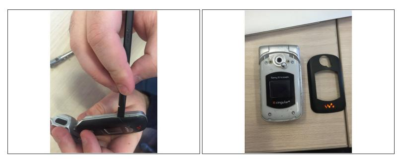
• Remove the front plate from the phone by using the prying tool.
