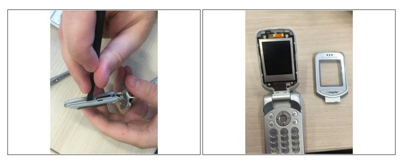
• Use the prying tool to separate the two parts of the top of the phone
