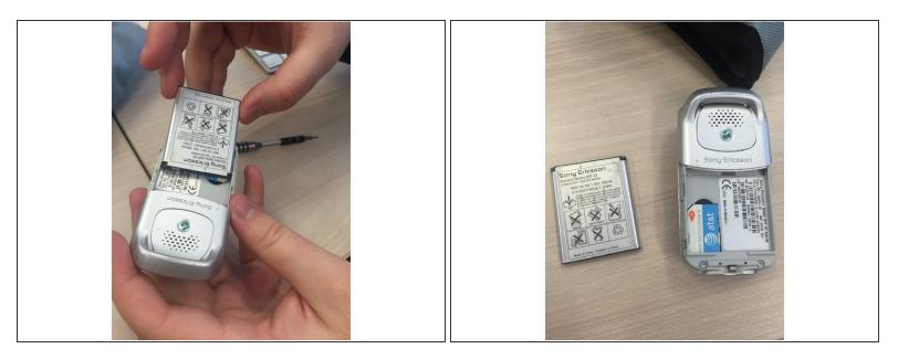
• Now, remove the battery from the phone by gently prying the battery out.
