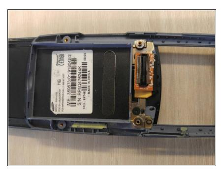
Peel off the black strip to expose two screws. Remove these.
