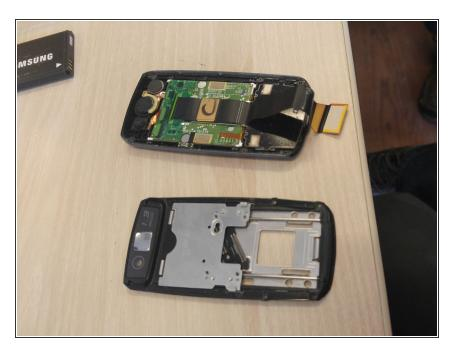
Use a Phillips head screwdriver to remove the four screws on the back of the screen.
