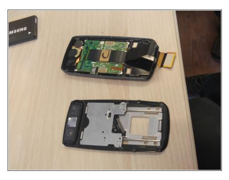
Once you have exposed the circuit board, peel off the green tape at the bottom. This will allow the removal of the screen.
