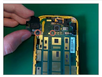
Remove two black Phillips head screws and remove the back speaker assembly.
