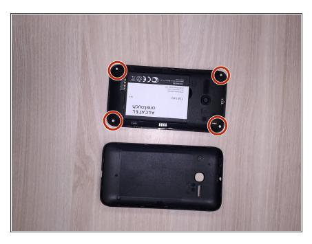
Using a J000 screwdriver, remove the four screws from the four corners of the back of the phone body. Keep the screws together and set aside.
