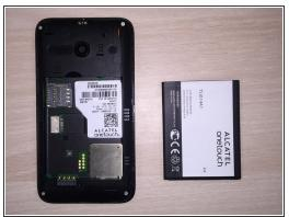
Remove battery from the back of device by prying the spudger underneath the battery, via the semicircular indentation at the top of the battery pack
