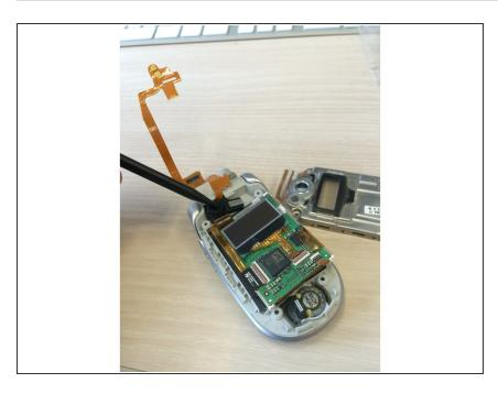
Insert black spudger beneath circuit board to pry it from phone screen.
