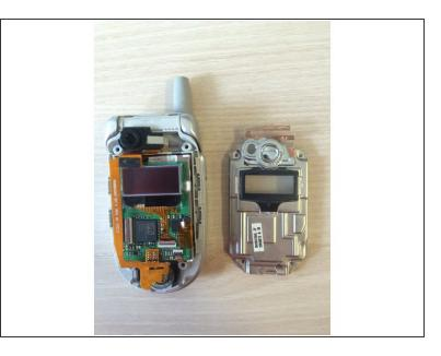
Use plastic opening tool to to separate inner metal cover from the circuit board. Apply pressure to remove the piece.
