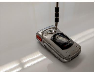
Use the T6 Torx screwdriver to remove the four screws.
